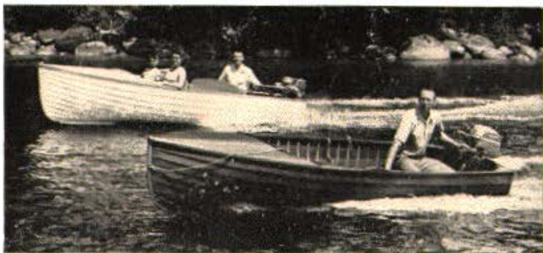
15 ft. Lapstrake Outboard — 22 H.P. Motor — Background 13 3/4 ft. Lapstrake Decked — 10 H.P. Motor — Foreground
